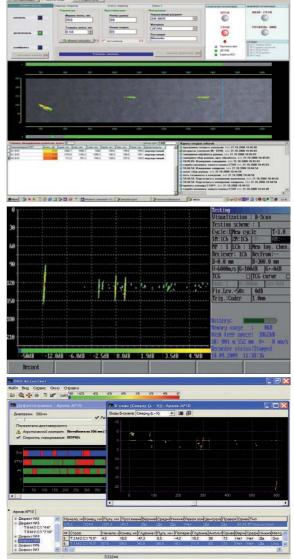
OKO-22M-UT represents a compact module, which can be easily installed on both mobile systems of sheets testing and special industrial cabinets of large-sized automated systems. The number of channels integrated into one system structure can amount up to 200. High performance of pulser and OKO-22M-UT board receiver allows to ensure the generation and receipt of short pulses, with the possibility to minimize the dead zones at the sheet surfaces as much as possible.
