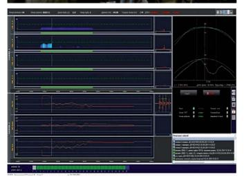
The on-line weld profile monitoring system provides the internal and external profiles of the tested weld and HAZ area along with its thickness. The material thickness and profile alarms notify the operator when the product does not meet calibration parameters. Extremely hard environment conditions are applied by IP64 OKO-22M-UT blocks. Fast Software provides high-speed tube testing with 10 channels simultaneously.
