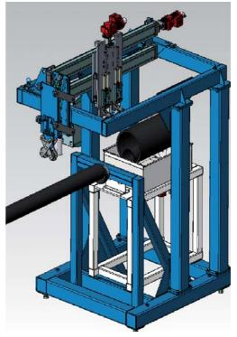
OKO-22M-UT is a high-speed waveform capturing platform and includes flexible signal gating, intended for streamlining hig-volume data acquisition tasks. This brand-new ultrasonic technique as well as OeM-ultrasonic board in connection with scan mechanics gives high in-line productivity. OKO-22M-UT guarantees an easy integration, especially in automated hot-rolling production cycles for a continuously running 100% UT inspection, including automatic registration and data storing.
