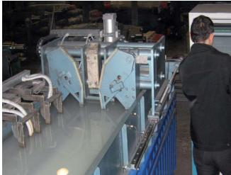
OKO-22M-UT is the best for immersion ultrasonic testing of axles and shafts for the presence of internal discontinuities and changes in attenuation of ultrasonic vibrations in the part material. The system applies all obligatory and additional techniques of acceptance ultrasonic testing, to every testing part, according to international standarts. Specialized Software presents such testing results: amplitude, depth, coordinates and conditional defects sizes.
